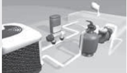
**GAS TRAP:** The cell must be positioned in such a way as to provide a gas trap. The bottom of the cell must be above the top surface of the pipe from the previous piece of equipment, as per the below diagram.
