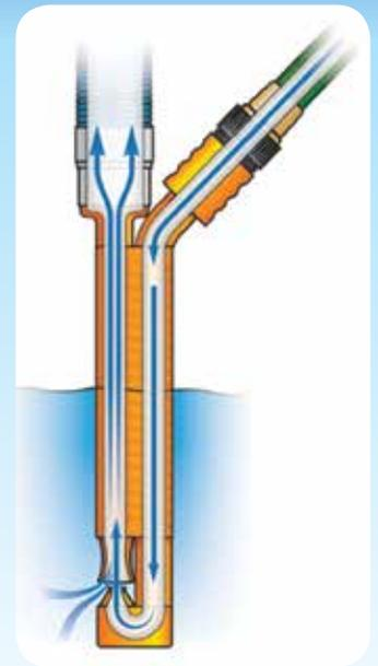
By using the pressure from the garden hose, this simple but effective submersible pump will drain up to 4,500 litres of water per hour with optimal water pressure. The average output is between 3,025 to 3,400 litres of water per hour.
